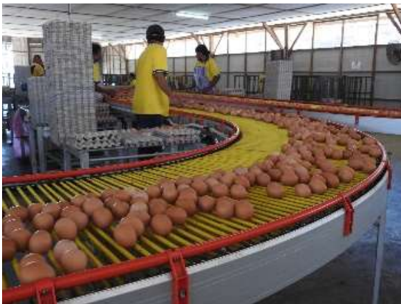
Automated conveyor belts from chicken houses to eggstore for collection of eggs
